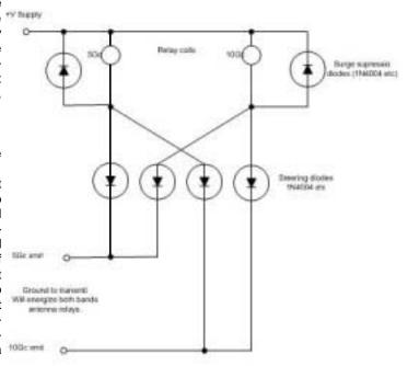
each transverters antenna relay. If your transverters are in separate boxes, you'll need to bring the cold end of the relay and the line that used to go there out to a little box or board between. Using feedthrus on each will be the cleanest way. 73, Joe AA3GN
